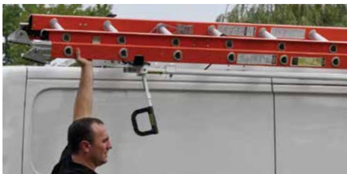
Lift ladder off the rear bracket.
